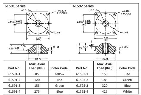
Deflection at Maximum Load = 0.25" Radial Stiffness = 2.5 x Axial Stiffness
