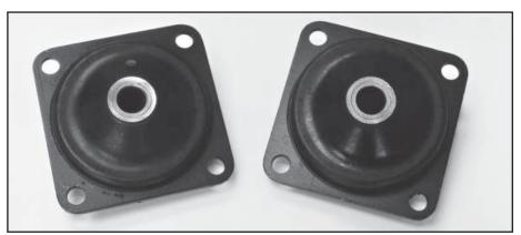
Tech Products' Heavy Duty Plate Mounts provide excellent vibration isolation for applications where a low natural frequency is required. At rated loads, these mounts provide a natural frequency below 7 Hz. Typical applications include gas and diesel engines, generator sets, pumps, compressors, and many other types of mobile equipment.
